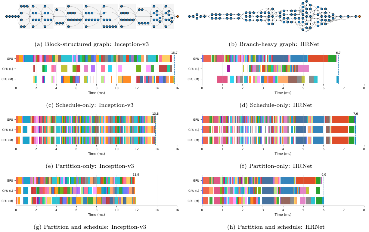
Figure 2: Branch-structured models on OnePlus 11 phone. Inception-v3 has limited branch-level parallelism, so partitioning can use idle devices. HRNet exposes more ready operators, so partition-only execution can block useful inter-operator parallelism. Joint partitioning and scheduling balance these effects.
